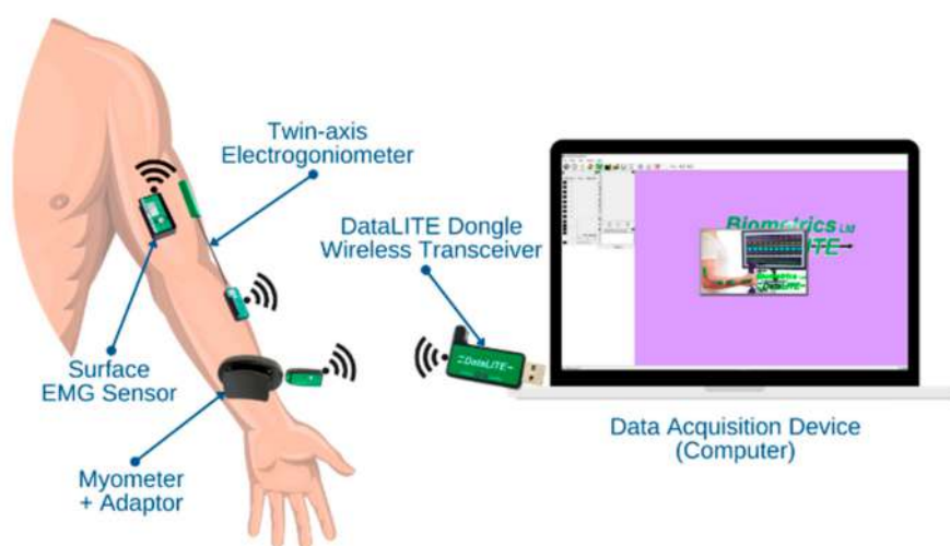
Figure 3. Connectivity between the DataLITE sensors and the computer.
