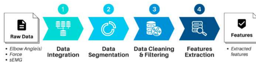
Figure 6. Data preprocessing stages to convert the raw data into extracted features.
